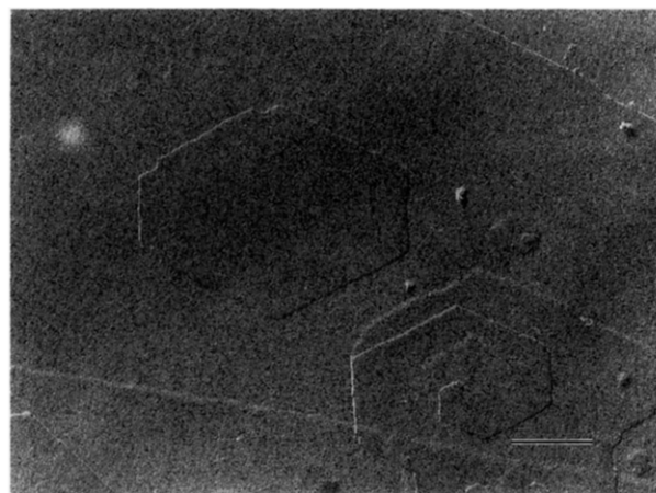
Figure 4. Terrace-like PBS single crystal. The single crystals were grown at 65 °C from 0.01 wt % o -dichlorobenzene and shadowed with Pt to increase the contrast for TEM (bar: 0.4 \mu\text{m} ).
